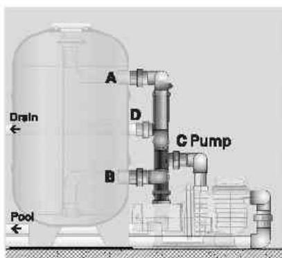
Besgo valves (DN65 / DN80 / DN100 / DN125) should be attached to the wall on site using pipe clamps.
